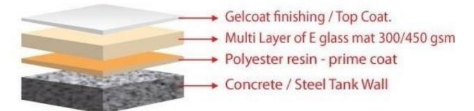
GRP Lining is a permanent layer coating process for Concrete Tanks to prevent leakage and water absorption, GRP Lining for Underground Concrete water tanks prevents algae and fungal growth. GRP Lining is permanent layer coating process, and will last for a lifetime. GRP lined tanks are suitable for storage of potable water as we are using the same water Tank manufacturing materials for GRP Lining.
