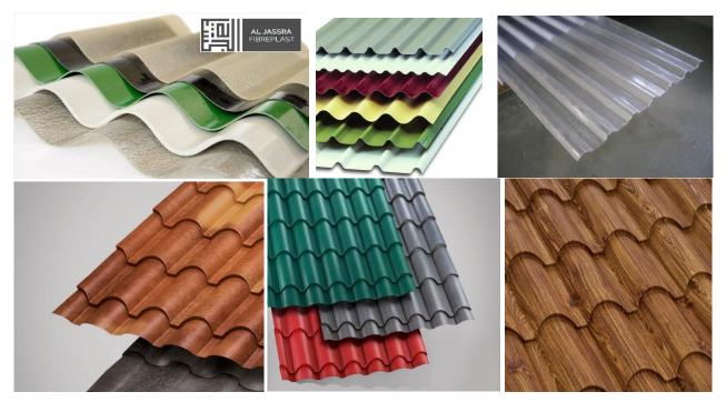
GRP roof and cladding sheets offer a high quality and flexible roof sheeting solution with a long lifespan. Made from high quality polyester resins and glassfibre reinforcements, they add high mechanical strength properties to the product. Sheets can be made to order up to 13 meters long and from 1.5mm to 6mm thick according required application and profile.
