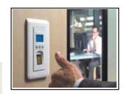
Access Control System restricts the access to a particular area to certain people either using biometric reader or by proximity cards. The main parts of the access control system includes reader Proximity or biometric type (Fingerprint recognition, Iris Recognition, Face recognition), Electromagnetic lock, Exit push Button, Access controller. The system can also be used for time attendance also
