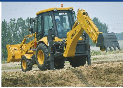
SDLG Backhoe Loader is remarkably versatile, whether you are using the loader or the excavator, it has the power and maneuverability to handle most jobs in this weight class. The Weichai engine together with the efficient SDLG hydraulic system provides 60 kN breakout force.
