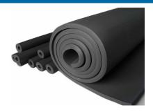
The Elastomeric Foam Pipe Insulation is for Refrigeration, HVAC and Plumbing. The moisture-resistant characteristics make it especially valuable on chilled-water and refrigeration piping where condensation might otherwise soak through fibrous types of insulations, significantly degrading their thermal performance, leaving them susceptible to fungal growth and ultimately
