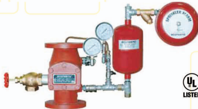
Alarm Check Valve assembly complete with constant pressure trim, retard chamber and water motor alarm gong
